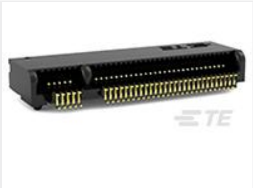
TE 产品编号2199119-8 M.2 0.5PITCH 3.2H KEY A 15U" AU
