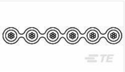
TE 产品编号4-1437356-9 171-14G=14P 28AWG STRAND PVC 1
