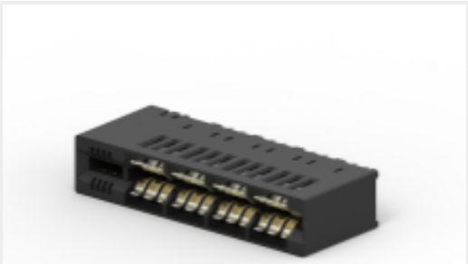
TE 产品编号2212112-1 MULTI-BEAM CE 2X4 PWR X 2X4 SIGNAL
