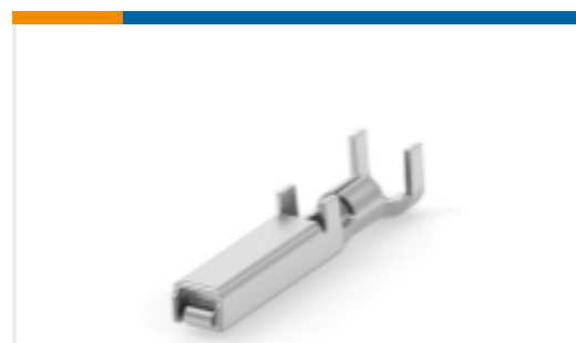
TE 产品编号917511-2 Contact: Component To Wire; 15A, 28-14 wire size
