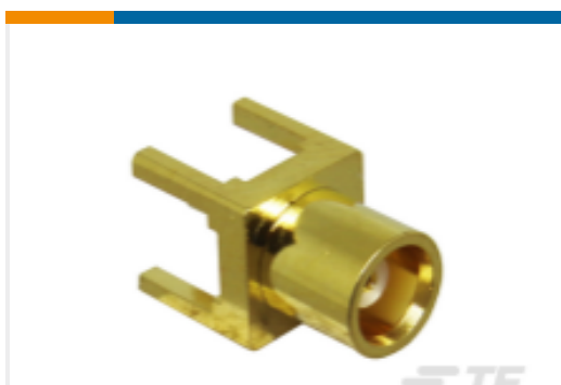
TE 产品编号CONMCX001 MCX Jack 50 Ohm PCB Through Hole
