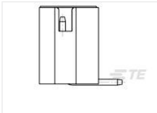
TE 产品编号2-1775470-2 HPI CONN., 2.0MM, V/T, SMT, 2P, GF
