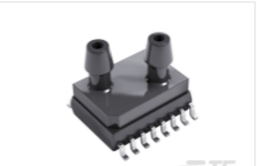
TE 产品编号9541-020C-D-C-3-S PRESSURE I2C 0.3PSID SO16
