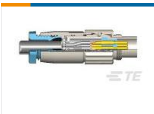
TE 产品编号1-1437719-1 T01-0540-P03-MALE PLUG CONNECTOR-CRIMP
