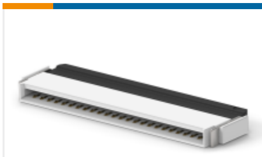
TE 产品编号2-2328702-4 24 PIN 0.5mm P FPC CONN, BACK FLIP LOCK
