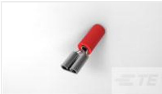
TE 产品编号640917-2 RECEPT,PIDG FASTON 22-18 187
