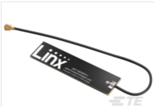
TE 产品编号L9000231-01 Antenna WIFI6 2.4/5/6 GHz RPC MHF4 100
