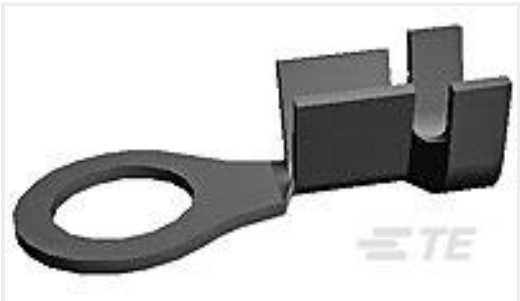
TE 产品编号63698-1 RING,M4, DIA 4.39,16-12,TPBR
