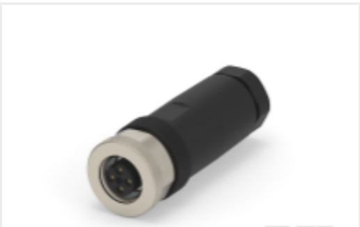
TE 产品编号 T4110402041-000 M12,FEMALE,STRAIGHT,B CODE,4P, PG9,GOLD
