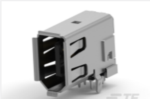
TE 产品编号2232261-2 1394_A RECEPTACLE UP RIGHT RA THRU HOLE
