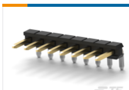
TE 产品编号2842111-8 8P,2MM,BRK HDR,SRRT,2.8,0.38AU,TB
