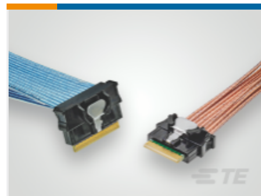
TE 产品编号2821747-1 SLIVER C/A, 50P, STR TO STR, 10GHZ, 100OHM
