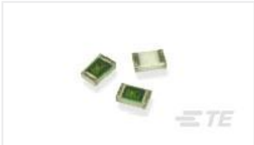
TE 产品编号6-2176091-7 RP 2A 0.25W 287R 0.1% 25PPM 1K RL
