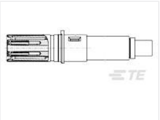
TE 产品编号1445693-3 SOCKET CONTACT,QUADRAX,SZ8,RR
