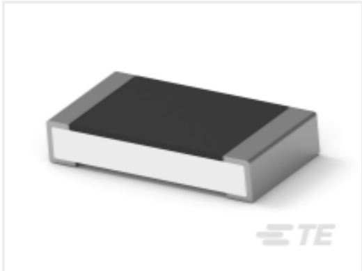
TE 产品编号6-2176389-0 RQ 1206 442R 0.1% 10PPM 5K RL
