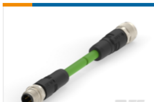
TE 产品编号TAD14541111-002 M12D4-MS-FS-PVC-22SH-TYPE B GREEN-1.0M
