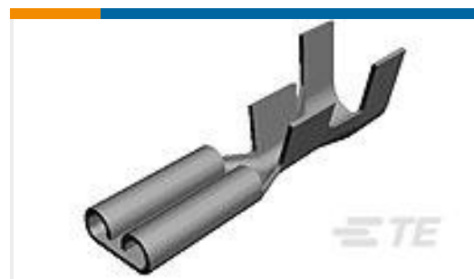
TE 产品编号60635-3 250 FASTON REC 14-10 AWG BR
