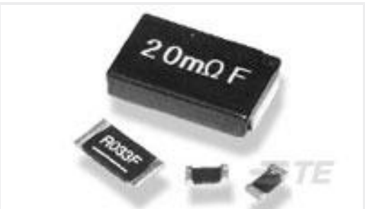
TE 产品编号2-1879378-4 TLR 2512 3.0W R002 1% 50PPM 2K RL
