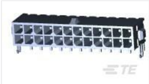
TE 产品编号5-794677-4 24POS MICRO MNL ASSY,R/A,THRU
