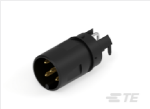
TE 产品编号225251-E M12 MALE, A CODE, RA, 5P THR REAR MOUNT
