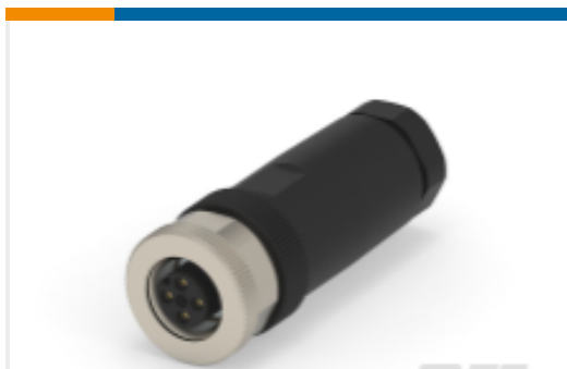
TE 产品编号T4110002041-000 M12,FEMALE,STRAIGHT,A CODE,4P, PG9,GOLD
