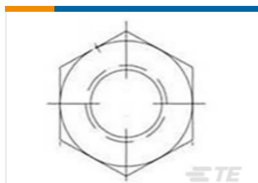
TE 产品编号1-328690-2 JAM NUT, GOLD PLATED
