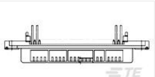
TE 产品编号5552241-1 ASSY, RCPT, 36 POS, EDGE MTG
