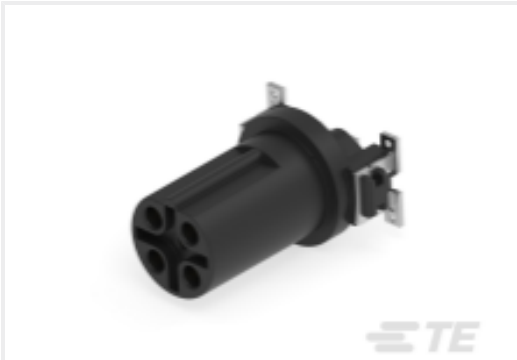
TE 产品编号454951-E M12 FEMALE, B CODE, 5P, 17MM SMT
