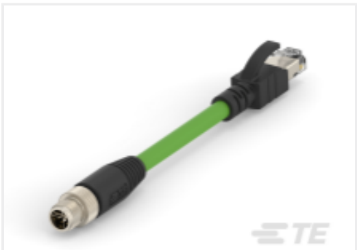
TE 产品编号CAT-SI113-M1ZA M12 X-code 8pin Male to RJ45 Cable Assembly, Cat6A Polyurethane 26AWG Shielded
