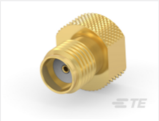
TE 产品编号2467941-1 RF TERMINATOR SMA JACK 18 GHZ 2W GOLD
