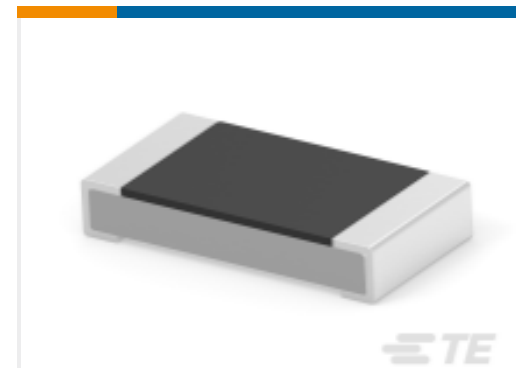
TE 产品编号2-2176392-9 RQ 1206 261K 0.1% 10PPM 5K RL
