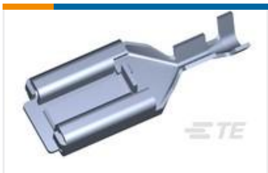
TE 产品编号368037-2 PL 250 REC 0.30-0.56MM2 0.40X21.0PRE-TIN
