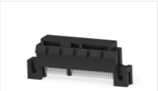
TE 产品编号2-2387405-2 PCIEG4,SMT,STRADDLE,64POS,30u", O/E
