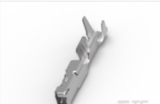
TE 产品编号2098762-4 Contact,female0.64, 22 AWG, CuNiSi, Sn
