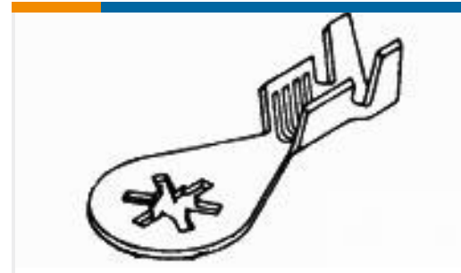
TE 产品编号640052-1 RING 18-14 AWG SST
