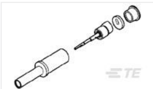
TE 产品编号1757624-1 SZ 8 COAX PIN,RG142,HEX CRIMP
