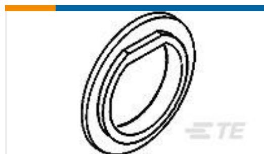
TE 产品编号330620 INSUL BUSHING BNC BLKHD PHEN
