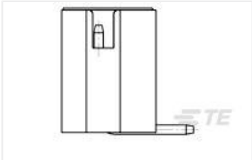
TE 产品编号2-1775470-3 HPI CONN., 2.0MM, V/T, SMT, 3P, GF
