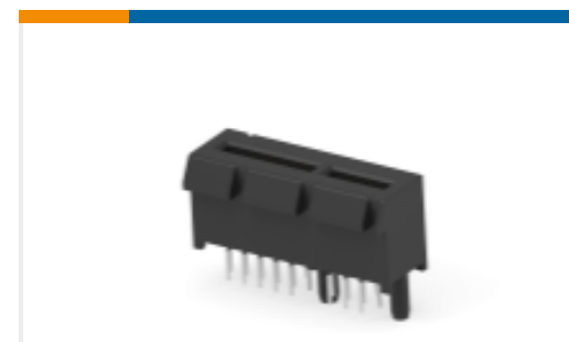
TE 产品编号3-2362375-1 PCIE GEN4, 36POS, G/F, DIP, 3.1mm TAIL
