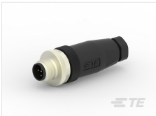
TE 产品编号T4111001051-000 M12,MALE,STRAIGHT,A CODE,5P, PG7,GOLD
