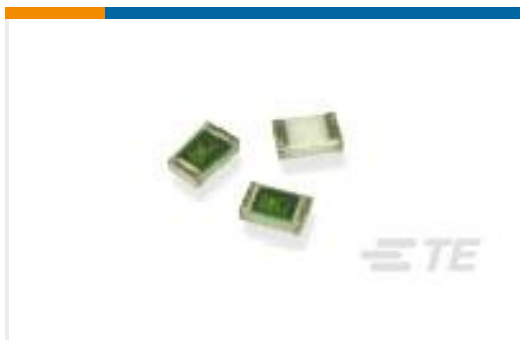
TE 产品编号2-1625868-7 RP 2A 0.25W 10R 0.1% 25PPM 1K RL
