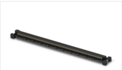
TE 产品编号2357739-1 16G,05FH,REC,220PIN,4H,Hard Tray
