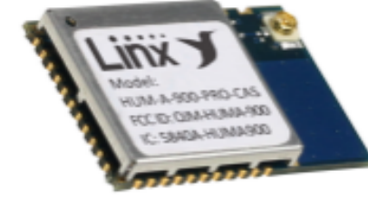
TE 产品编号HUM-A-900-PRO-CAS Module HUM-PRO-A 900MHz FHSS FM XCVR FCC
