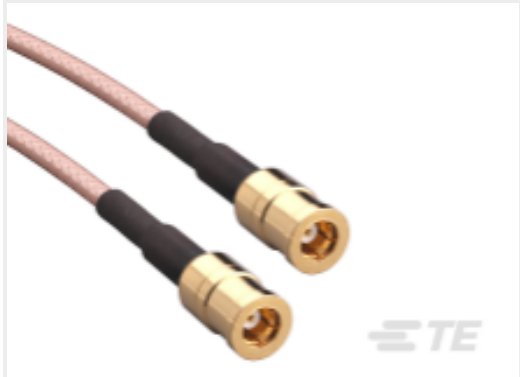
TE 产品编号CSE-SMBM-152-SMBM SMB to SMB 152mm RG316
