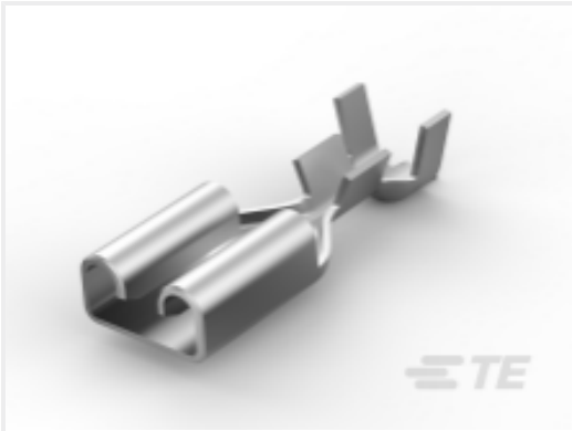
TE 产品编号2232974-1 187 FASTON,REC.,24-20 AWG,BR
