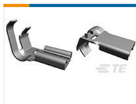
TE 产品编号 180430-2 250 FASTON, FLAG, REC., 20-16 AWG, TPBR
