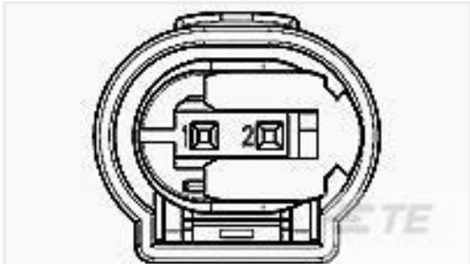
TE 产品编号2-967644-1 2POS MQS REC SEALED COD B
