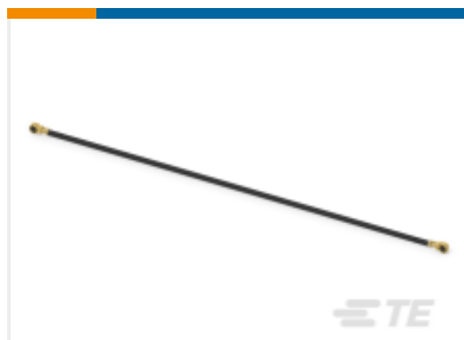
TE 产品编号1-2016698-6 RF CA,UMCC GEN4-GEN4,1.13MM CABLE,L200MM
