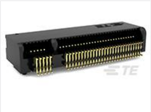
TE 产品编号2199230-5 M.2 0.5PITCH 4.2H KEY B 30U" AU
