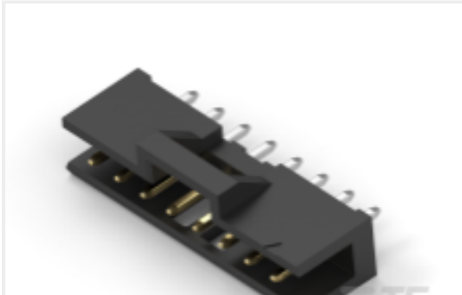
TE 产品编号2823402-8 8P,2MM,PL HDR,SRVT,2.8,0.76AU,TB
